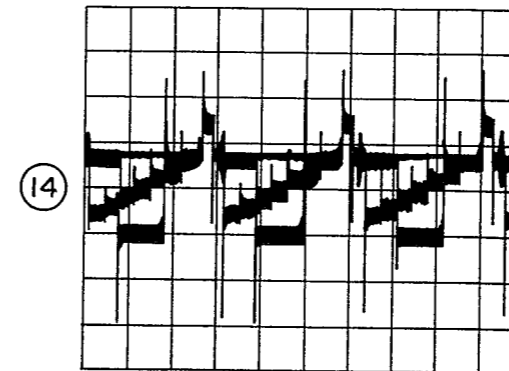
FIL411 OUT (PB) 20 \mu s/div. 100mV/div.
